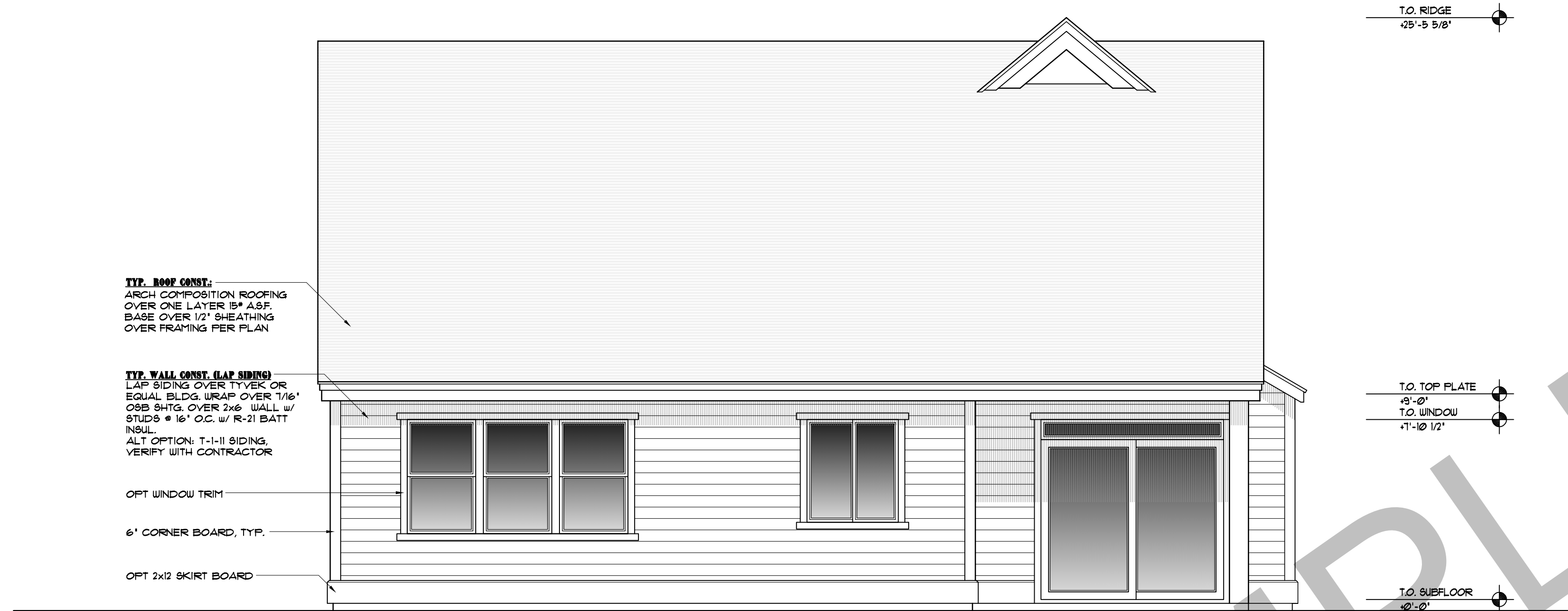
REAR ELEVATION SCALE: 1/4"-1'-0"
